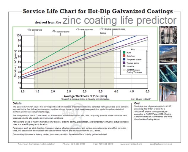
Figure: Projected service life of hot dipped galvanized structures
